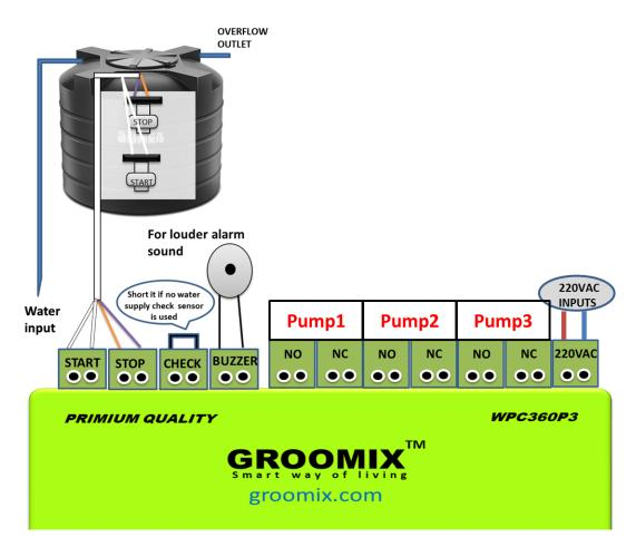
**CONNECTION DIAGRAM OF SENSORS AND PUMPS**
